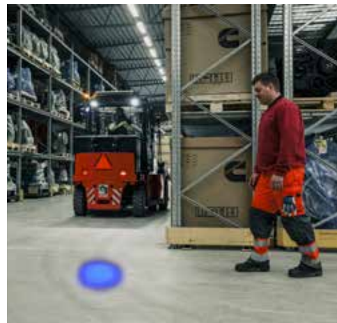
Blue safety light option. The blue safety light alerts people that the truck is approaching, reducing the risk of accidents.
