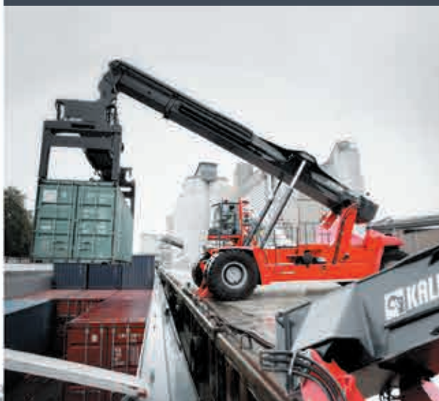
Trimodal / Barge handling.
