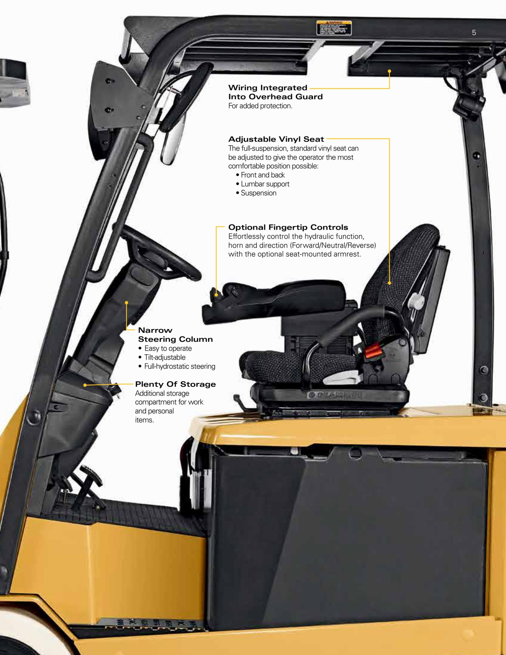
**Wiring Integrated Into Overhead Guard**
