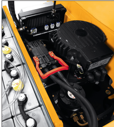
Drive and lift motor with AC technology
