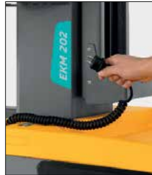
On-board charger with integrated spiral cable
