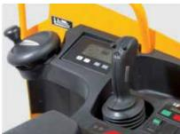
the operator with enhanced visibility. An All drive and lift functions are controlled by the multifunction joystick.
